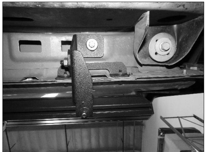
(Fig 4) Brackets mount to front location
