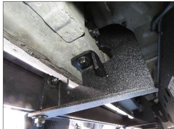
(Fig 4) Mounting bracket attached to the front mounting location
